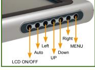
OSD Keypad is designed for AFL-15M/17M/19M
