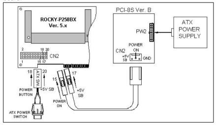
Connect the ATX power supply switch to the pin 18 (power button) and pin 20 (+5VSB) of CN2 (multi panel) on the board.
