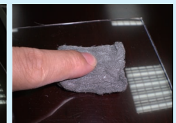
Abrasion Test (Steelwool #0000)
