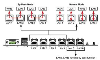
• The LAN Bypass feature could assure the connection to Internet, if the networking appliance platform fails.
