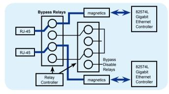
In "bypass" operation the RJ-45s are connected together such that they form a piece of wire.
